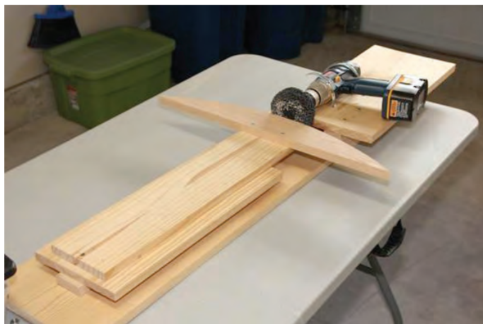
Pivoting jig for smoothing the circular bearing section using a hand drill and a grinding disc
