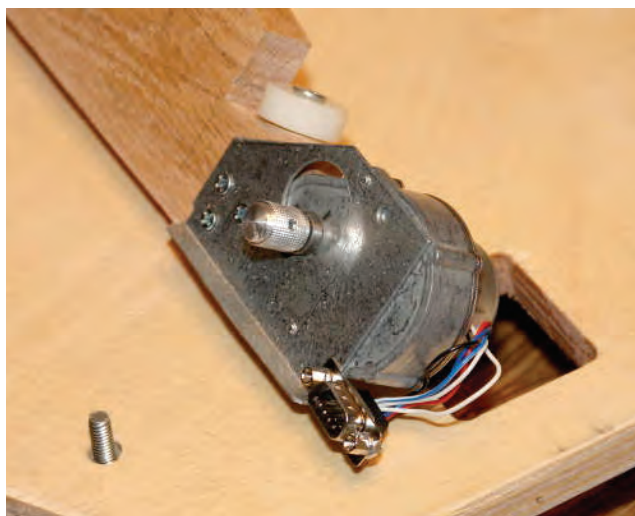
Close up of the drive motor mounted on the bearing support board.
