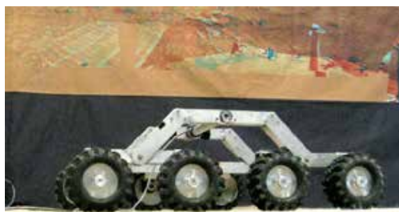
8-wheeled rover—developmental model for final Curiosity Rover
