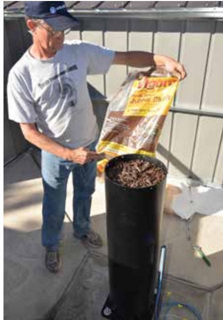
Figure 22: Recycled Tire Mulch to Dampen Vibration
