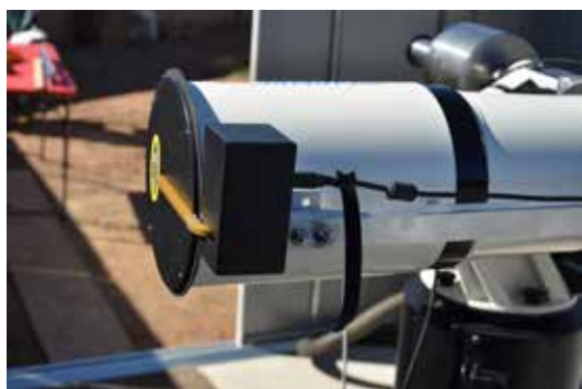
Figure 26: Flip Flat as a Dust Cover on a Homemade Rail
