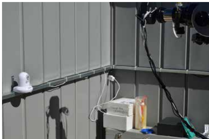
Figure 24: IP Camera for Observing Slews and Roof Status Inside the Observatory
