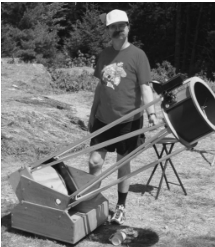
John Stewart and his 12.5-inch diameter homemade Dobsonian. He made the mirror in the NCA mirror-making workshop here in DC.
