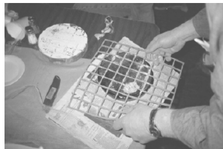
Don Surles getting ready to press the channels into a pitch lap. (Photo by the author)
