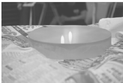
Grazing reflection of light bulbs in a fine-ground mirror. (Photo by the author)
